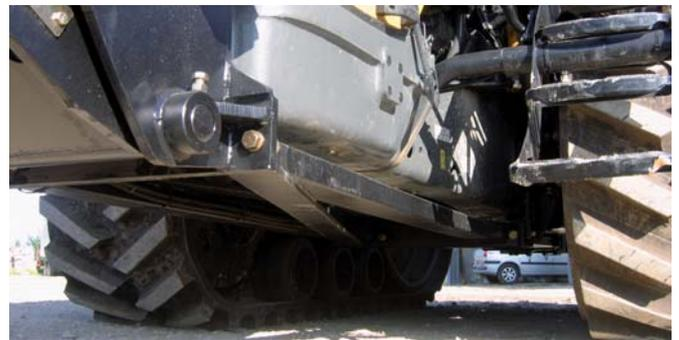
*The lower reinforcing frame maintains crop clearance*
