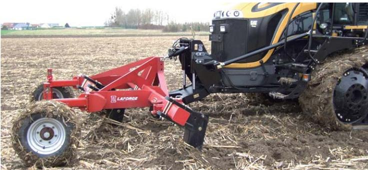
*HDIT front hitch with optional DYNA CONTOUR<sup>®</sup> attached to a UNIPASS<sup>®</sup> front sub-soiler*
