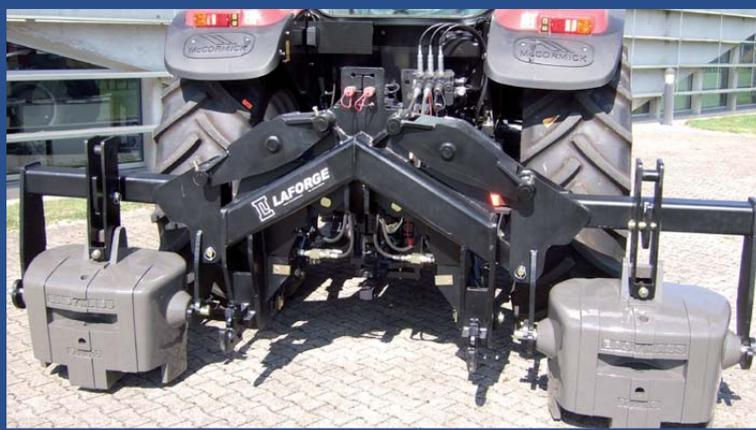
The 3-point hitch and the weights are lowered to adjust the amount of ballast weight.
