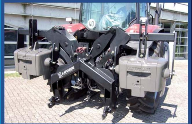
2-Stage FLEXIMASS® in raised position with the 3-point hitch lowered.
