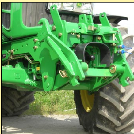
GreenLink Pr4.2 premium front hitch with optional LAFORGE front PTO
