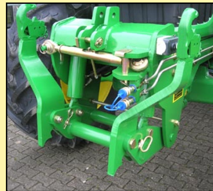
GreenLink St4.2 standard front hitch with optional remote hydraulic receptacles
