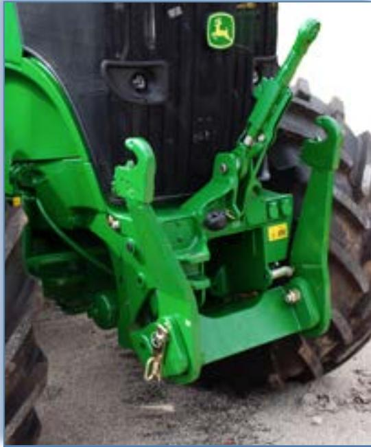
*Front Hitch GreenLinl® ST5.5/7R on 7R front hitch ready tractor*
