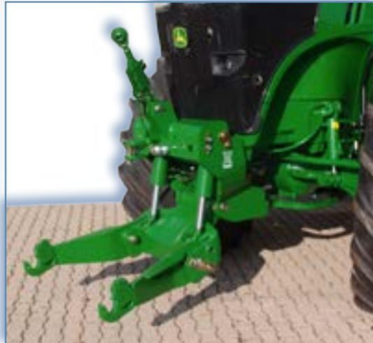
*Front Hitch GreenLink® PR5.5/7R on 7R non hitch ready tractor*
