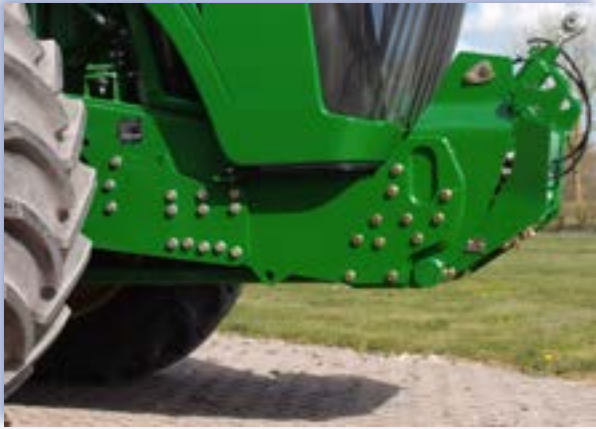
GreenLink® HD6/9R PowerFold® in folded up position with optional hydraulic center link
